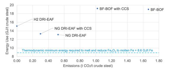
Figure 3. Energy-emissions tradespace for representative commercial and pilot ironmaking routes. *Source*: Own calculations, with assumptions based on values from IEA (2019) and Fan and Friedmann (2021). Thermodynamic minimum energy to produce molten iron is from Fruehan et al. (2000) and is roughly the energy needed to produce molten steel.
