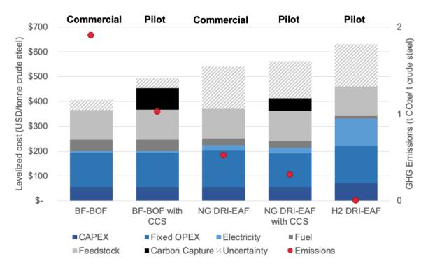
Figure 2. Levelized cost of steel for commercial and pilot routes as greenfield deployments with 3 c/kWh zero-carbon electricity. Emissions include Scope 1, Scope 2, and upstream coking process (Scope 3). *Source:* Own assumptions, based largely on IEA (2019) and Fan and Friedmann (2021). IEA (2019) The Future of Hydrogen, https://www.iea.org/reports/the-future-of-hydrogen. All rights reserved.
