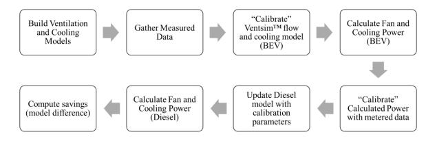
Figure 3: Adapted Calibration and Savings Determination Approach
