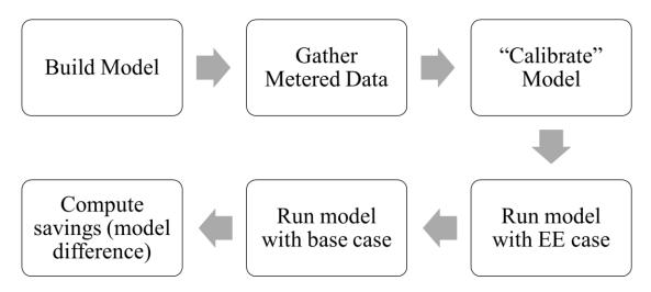
Figure 2: Basic "Option D" model calibration process
