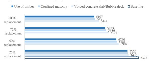
Figure 5: Reduction in GHG emissions in MtCO<sub>2</sub>/ton of cement by 2047- Demand-side interventions
