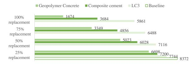
Figure 4: Reduction in GHG emissions in MtCO2/ton of cement by 2047- Supply-side interventions
