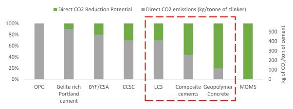
Figure 3: Emissions reduction potential of various low carbon alternative w.r.t OPC. Sources: (Scrivener, et al. 2018), (Hassan, Arif and Shariq 2019), (CII 2016), (Naqi and Jang 2019), (Sahu and Meyer 2020), (The American Ceramic Society 2011)
