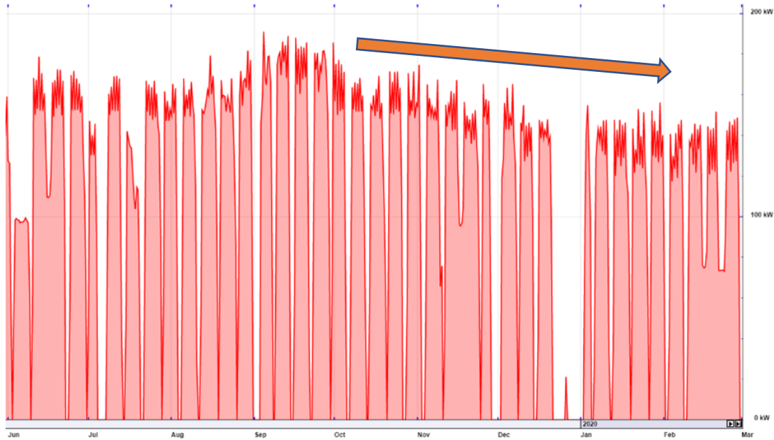
Figure 8. NSK's compressed air use from June 2019 through March 2020.
