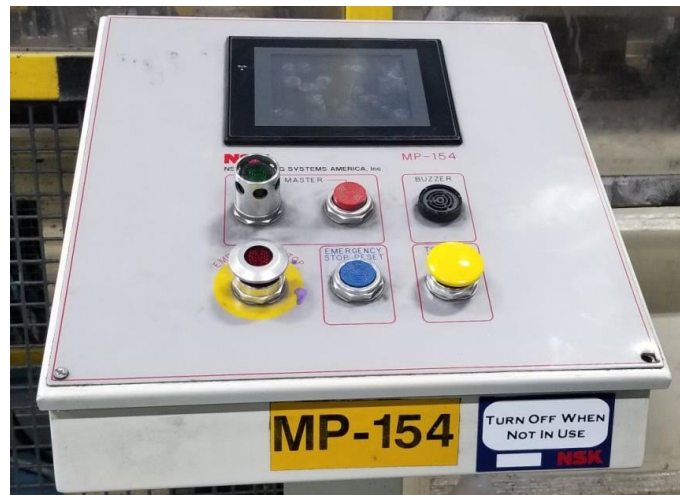
Figure 3. NSK identified if each machine can be turned off or not using stickers.
