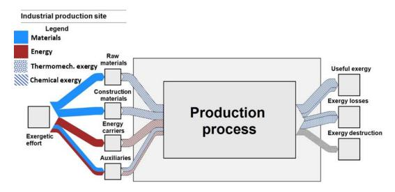
*Figure 5: Sankey diagram of an exergetic analysis of an industrial production site (Own figure)*
