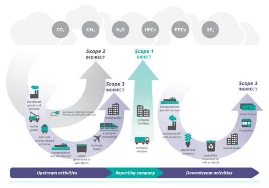
Figure 2: Overview of GHG Protocol scopes and emissions across the value chain. Source: GHG Protocol Initiative 2004
