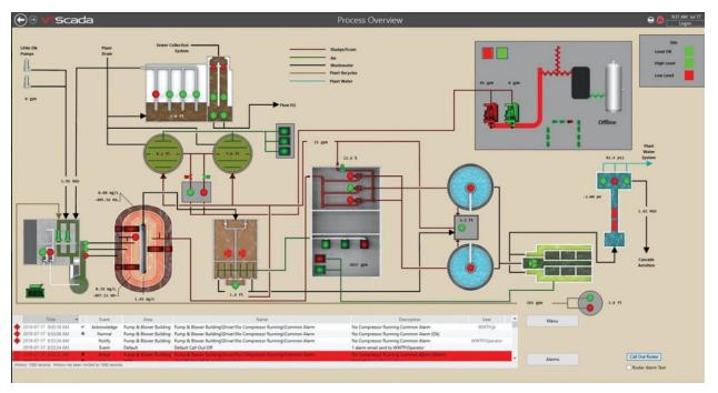
Figure 9. Example of SCADA Screen. Source: ESI
