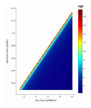
Figure 13. Payback period (PBP) of the modeled closed cycle, mechanical IHP vs. energy costs for the dairy process case study. Source this work.
