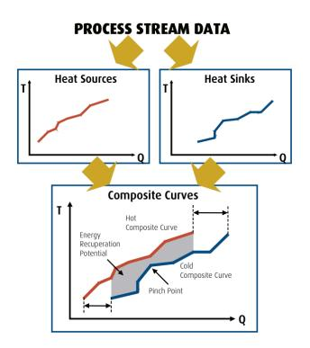
Figure. 8 – Explanation of pinch composite curves (NRCan, 2003)
