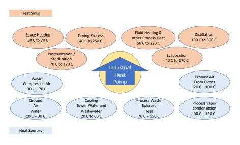
Figure 4 – Typical IHP heat sources and sinks. Source: this work.
