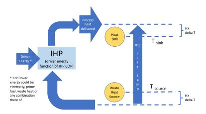
Figure 6 – Generic IHP diagram illustrating IHP lift temperature, T<sub>source</sub> and T<sub>sink</sub>
