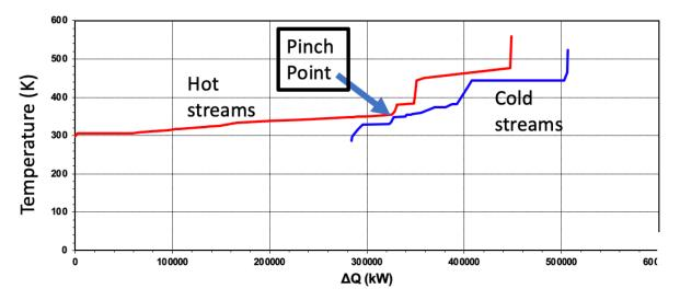
Figure 9. Pinch analysis for hot and cold streams for ethylene; quench water (hot stream, heat source) pumping heat to the boiler used to separate propylene (cold stream, heat sink). Data source: Franke 2021
